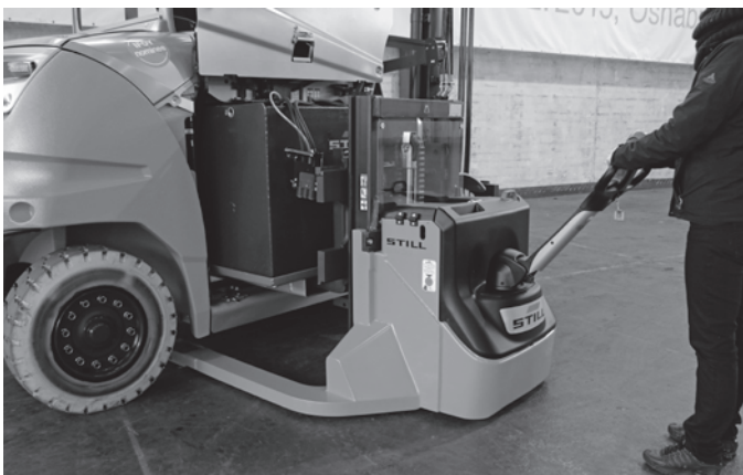
Fast battery change with ECU 30 high lift truck
