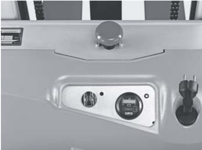
Everything in view at all times thanks to LED display with battery charge display and operating hours counter
