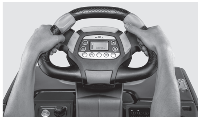
Thanks to the height-adjustable STILL Easy Drive steering wheel, all functions can be operated with ergonomic controls by right- and left-handed operators without changing grip 3
